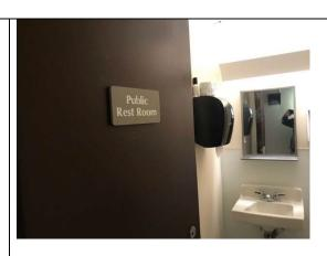
Relocate all movable fixtures to provide the maximum amount of barrier removal. Otherwise, this room will have to be reconstructed to gain sufficient space to make accessible under 2010 Standards.
