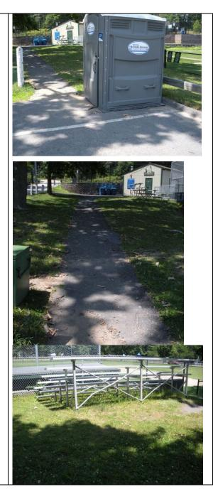
The complete lack of any accessible routes on this site will require a comprehensive master plan and design effort. It will be difficult to attempt to construct piecemeal improvements without the risk of having to remove them at a later date. 3 The sidewalk on the right-of way is 206 deteriorated and lacks the width to provide any site connectivity between the tennis/basketball courts and the parking/restrooms or other site elements.
